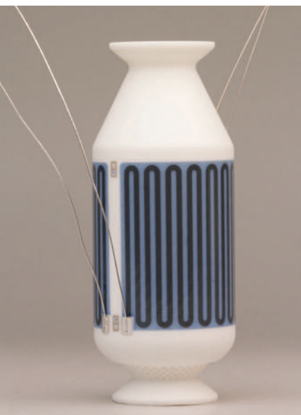
Reactor including electrical contacting.
